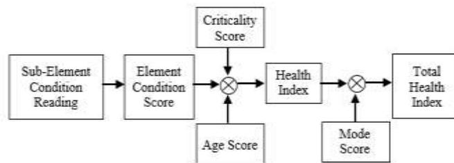
**Figure 3** Process Flow For Determining Health Index Of Power Transmission Lines And Cables. Adapted From [12]
