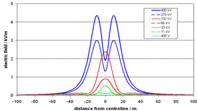
**Figure 3** Regular range of for power transmission line with different voltages [13].
