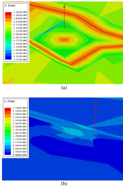
**Figure 5 (a)** Electric field simulation of parallel plate's harvester; **(b)** Electric field simulation of hollow cylindrical harvester.
