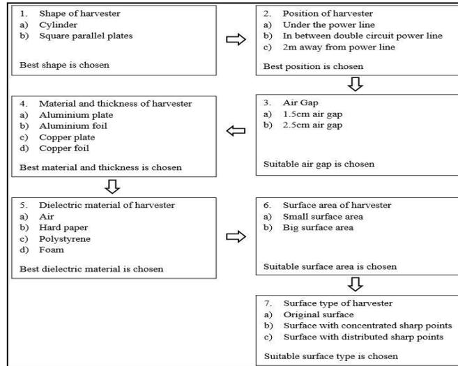
**Figure 1** The stages of forming an efficient EFEH
