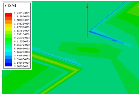
**Figure 8** Electric field simulation of parallel plates with foam, polystyrene and hard paper as dielectric material.
