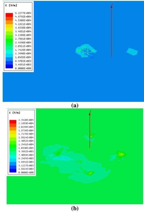
**Figure 10** (a) Electric field simulation of parallel plate’s harvester with concentrated sharp points; (b) Electric field simulation of parallel plate’s harvester with distributed sharp points.
