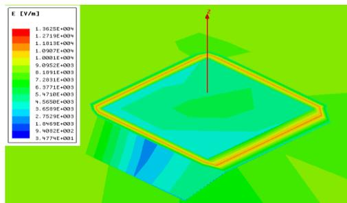
**Figure 9** Electric field simulation of bigger surface area parallel plates with foam as Dielectric Material
