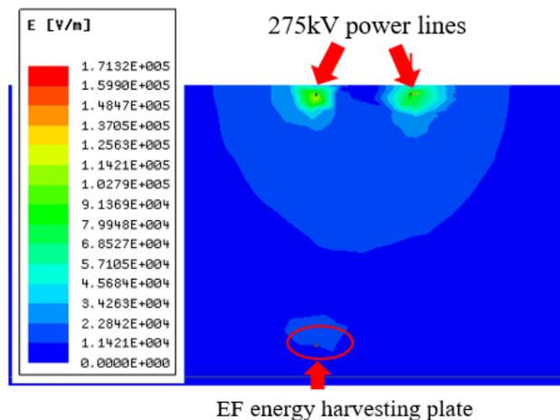
**Figure 2** Simulation of electric field generated around 275kV power line using ANSYS Maxwell software
