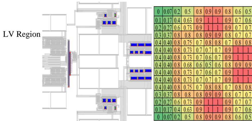
**Figure 6** Full Chip Thermal Profile Showing LV Area on the Left that is Causing Thermal Gradient Issue.
