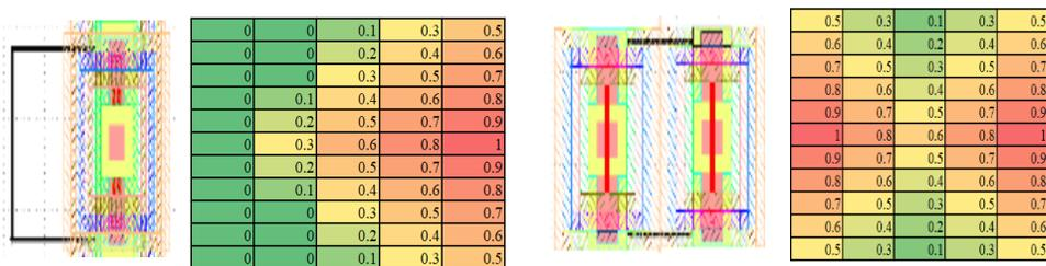
**Figure 5** Heat Map Showing Heat Source Distribution and Thermal Gradient Violations (Left) and (Right) After Smoothing.
