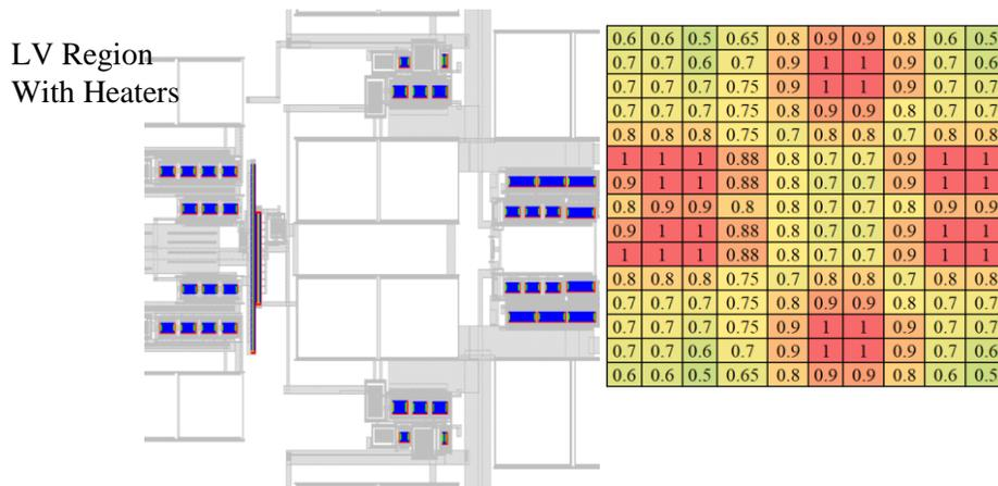
**Figure 7** Full Chip Thermal Profile after Fixing Thermal Symmetry and Gradient Issues by Adding Heaters in LV Region
