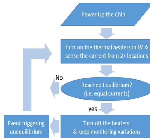
**Figure 2** Methodology of Operating Thermal
