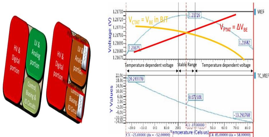
**Figure 1** Tradition Full Chip Heat Map with No Heaters Showing Thermal skewness/gradient (left) and chip in equilibrium either after settling or incorporating heaters aiming for faster settling time and wider temperature compensation and stability range (right). Note: the color code used shows dark red as hot region and green as cold one.
